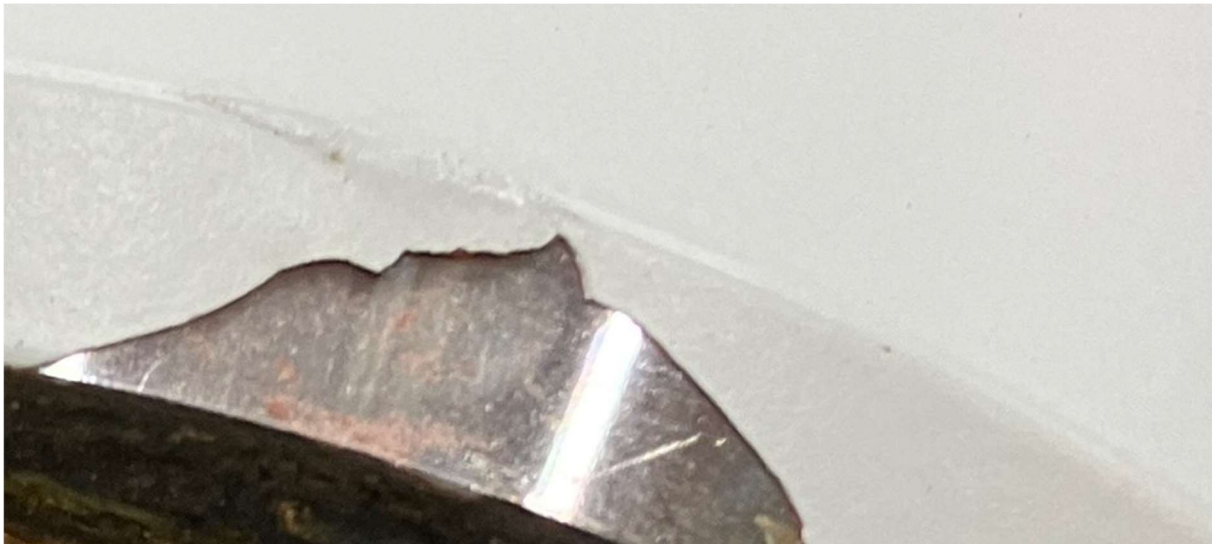
Picture 2 – Peeled painting from customer claim
